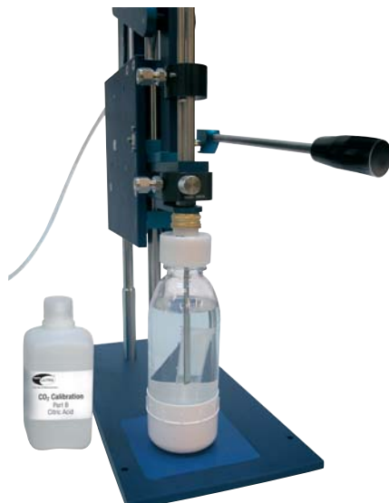
Figure 2: High precision CO 2 calibration kit.
